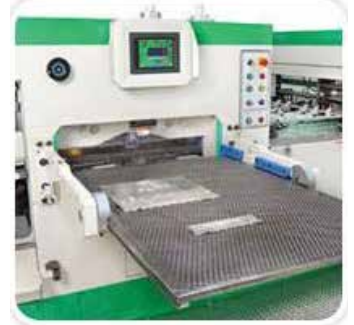
Heating Plate System
