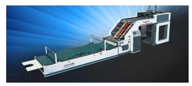
The machine is perfectly combined with the motion control system and the servo correction system. It uses multiple sets of highprecision photoelectric sensors to track and position the paper, and corrects the paper through the servo motor to achieve accurate positioning of the paper and the bottom paper. It has many advantages such as high speed, high precision, convenient operation, etc. It is an indispensable equipment for color printing and packaging users.
