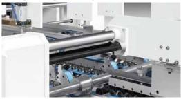
\* Automatic alignment system to correct the paper feeding, avoiding the paper going to sides.
