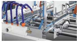
\* Pressure can be adjusted according to paper thickness. For flute E/C/B/A corrugated board, overlapping and jogger devices are equipped to ensure box gulling well. After kicker is set up, whatever speed the machine runs, the kicker can automatically follow, no need to reset it.
