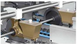
\* Lock-bottom assembly mechanism with high elastic hookers is of ideal design, fast and easy operation.
